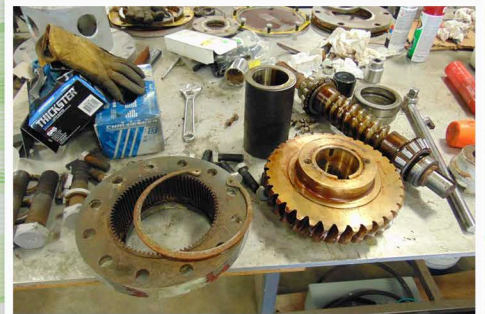
Ralston Afterbay Gate 5 hoist gearbox overhaul in progress
